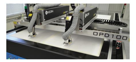
The OptiDual system is equipped with dual laser sources instantly doubling your laser cutting production. The KCAM laser software controls each laser independently allowing both lasers to be tuned to equal power. This feature ensures consistent cutting results from both lasers over the entire work area. The second laser can be disabled allowing full range of table motion for the master laser.
