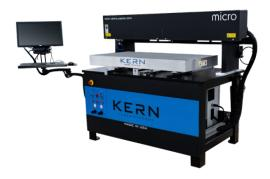
model and the Y axis is a moving table that increases the accuracy and speed while cutting. Like all Kern systems the MICRO is a turnkey package including the computer, software and downdraft vacuum system.
