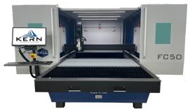
laser system include a pull-out processing table with an integrated downdraft vacuum table, parts collection drawer and convenient sheet metal hold down pins along the perimeter of the processing table. These new features are designed for enhanced efficiency and streamlined workflow in your workspace.
